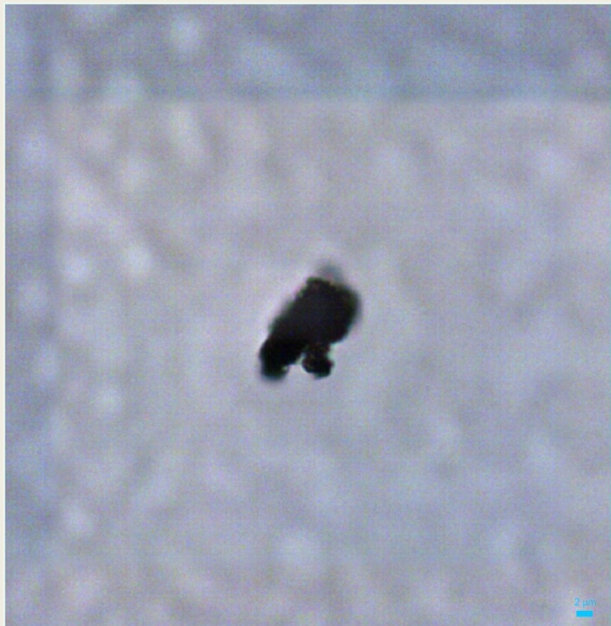
▲ Graphene-like particle image acquired with transmitted light and 100x objective
